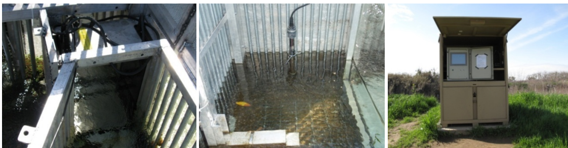
Figure 6. Left: Photograph of the Vaki Riverwatcher infrared scanner looking from upstream to downstream at the upstream side of the scanner plates. Center: Example of the riverwatcher camera and lights. Right: Tuolumne Weir Vaki Riverwatcher computer system and job box.
