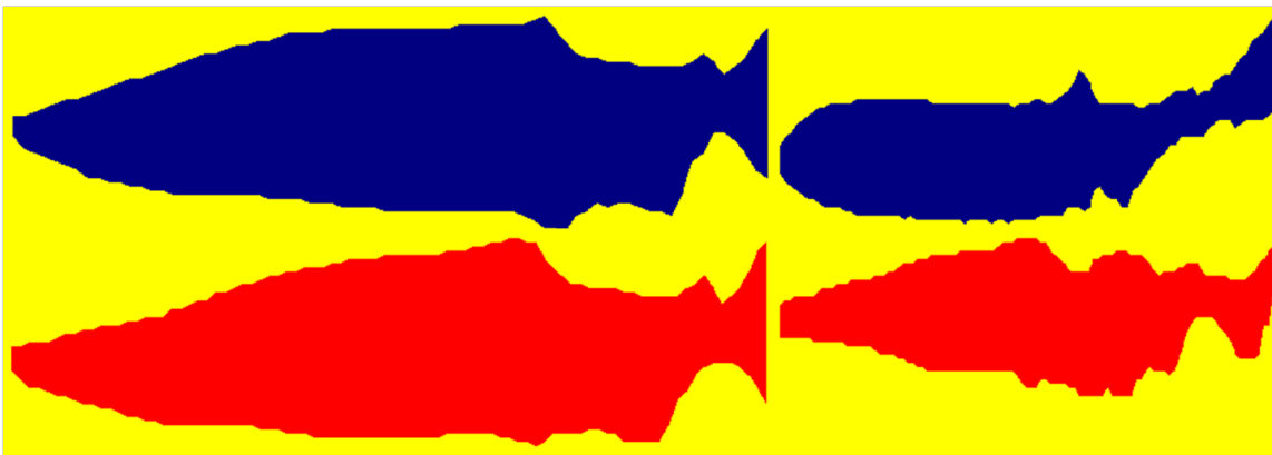
Figure 7. Example of silhouette images produced from both sets of scanner diodes (one image from one set of diodes is displayed in blue and the other is displayed in red). The left set of images is an example of a typical salmonid silhouette and the right set of images is an example of a poor salmonid silhouette.
